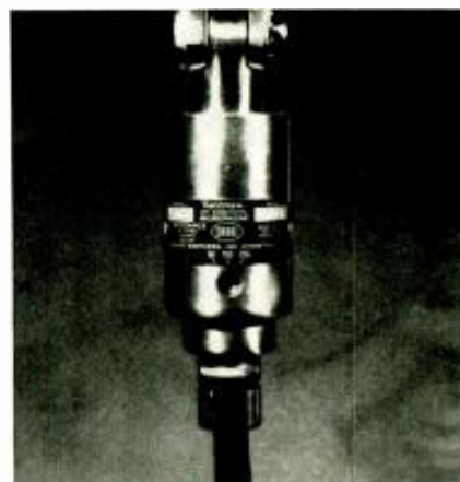
Impedance adjustment on the 330 is made by turning the screw mounted on the shock-proof base mount of the microphone.
